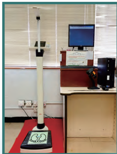
通過連接電腦和電子測距儀，把量度得到的身高和體重數據直接傳輸至電腦系統 Connection between computer system & Electronic Stadiometer to facilitate direct transmission of the body height and weight measurements to the computer system
